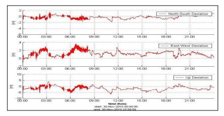
Figure 2: Deviation from the reference coordinate with GPS standalone
