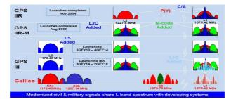
Figure 1: GPS Signal Modernization
